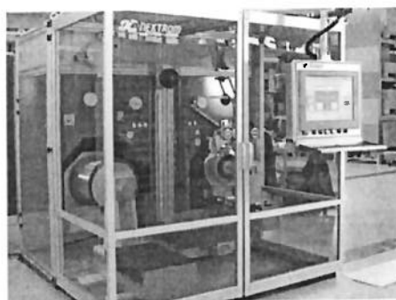
OFC 35 – PROOF TESTING AND REWINDING LINE Comprising a Testing Unit, a Pay-off and Take-up with Dancers
